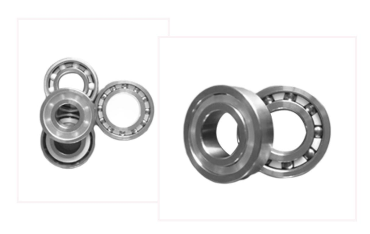
However, not like 440C or 420 stainless steel (higher carbon chromium martensitic stainless steel), AISI316L and SUS304 stainless steel (austenitic stainless steel) cannot be quenched as whole, bearings made out of AISI316L and SUS304 are not suitable for heavy load and high speed.
