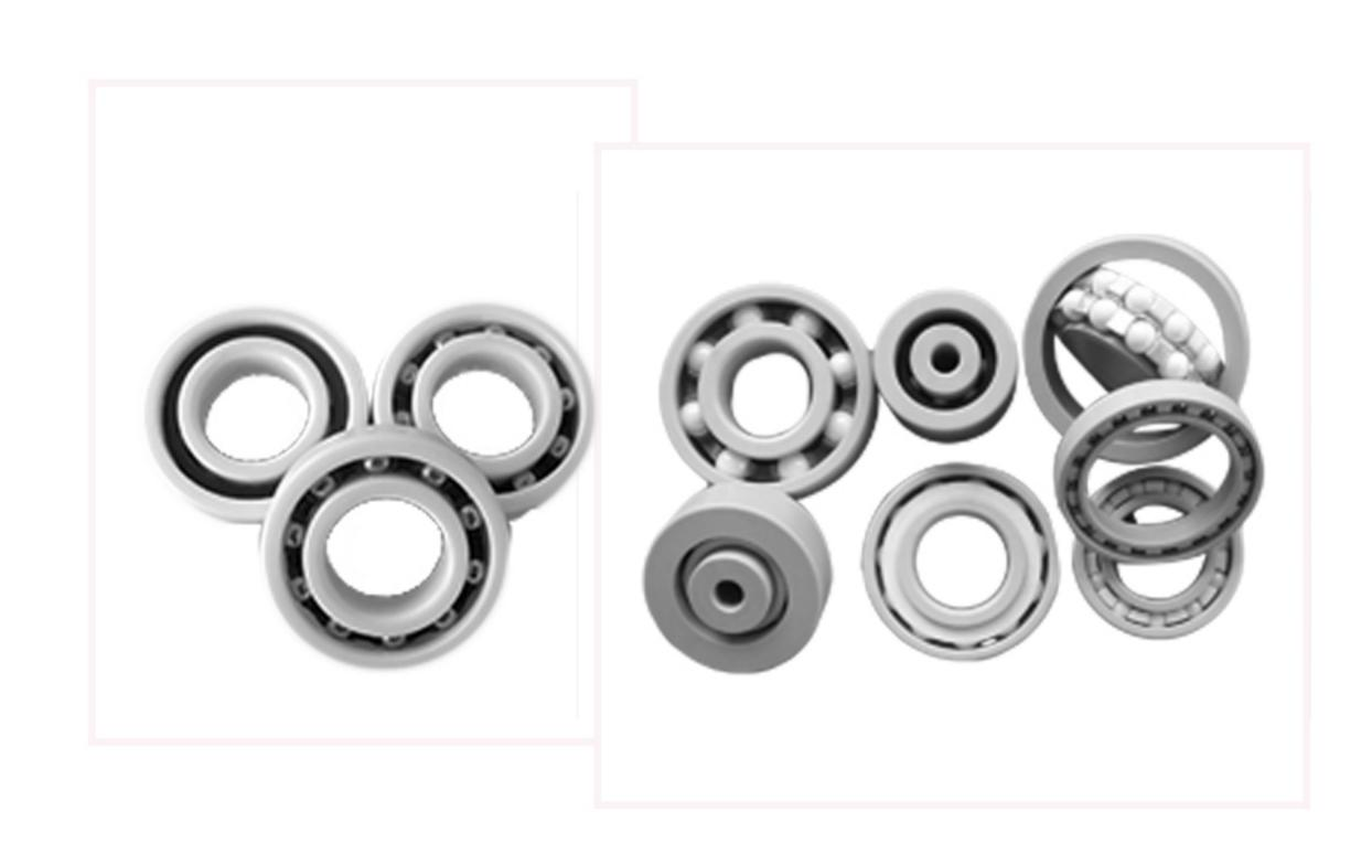
Plastic bearing made in POM is applied most extensively among all plastic bearings. In general, the inner and outer ring materials are made in POM or PA, cages are made in PA and the balls are made in glass, stainless steel or ceramic. These bearings are alkali resistant but not acid resistant.
