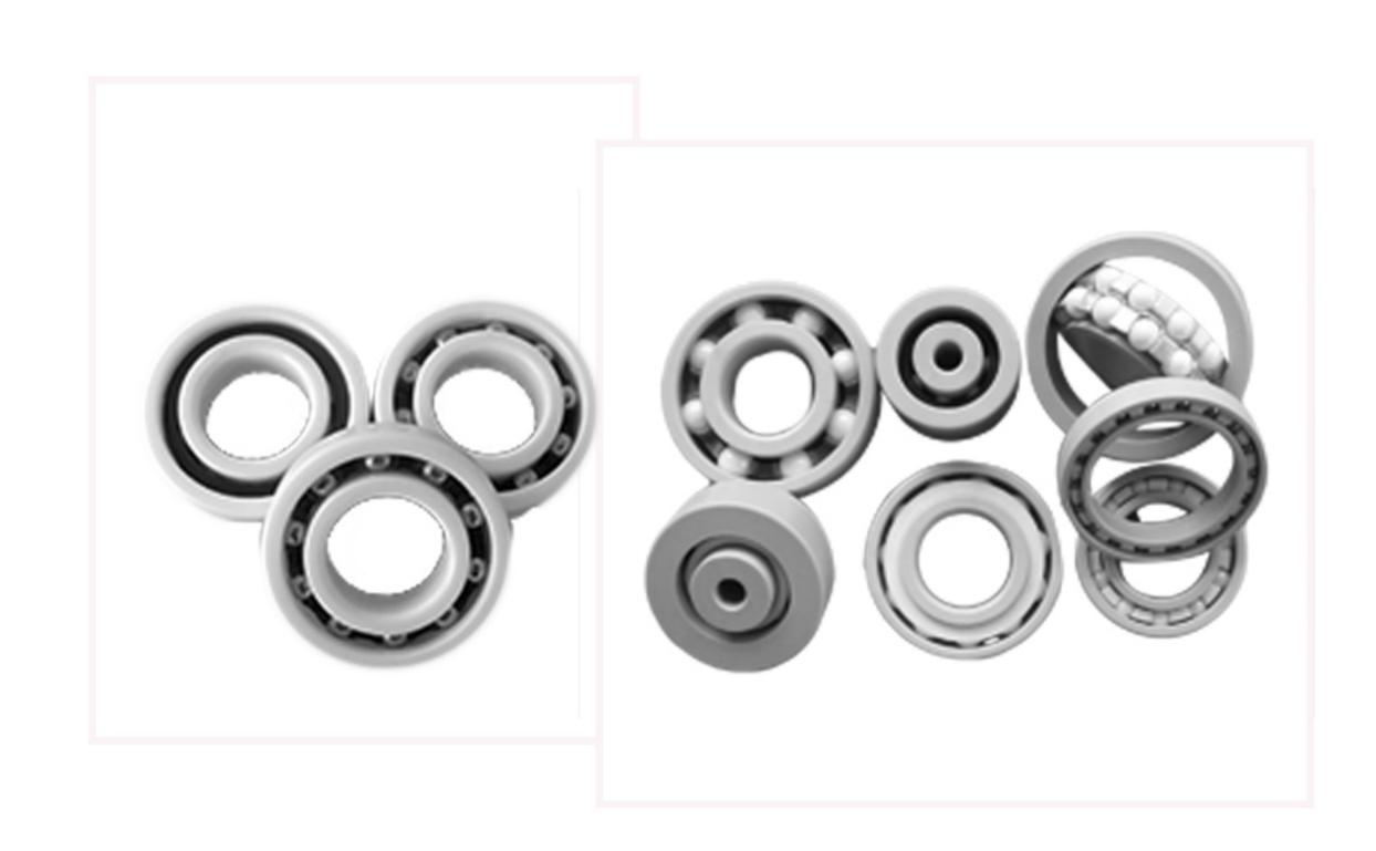
Plastic bearing made in POM is applied most extensively among all plastic bearings. In general, the inner and outer ring materials are made in POM or PA, cages are made in PA and the balls are made in glass, stainless steel or ceramic. These bearings are alkali resistant but not acid resistant.
